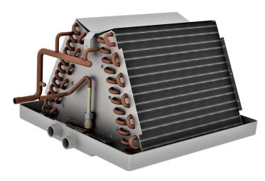
The **USM** series coil can be field installed into an air handler with sufficient space. A piston-type metering device is utilized for maximum flexibility. Optional R-22 or R-410A field installed TXV kits are available.
